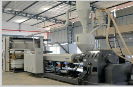
Tape Plant having capacity to produce 14 MT PP Tapes per day
